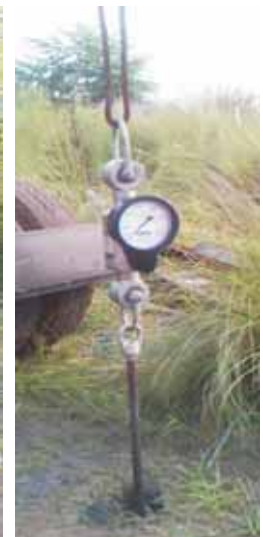
Simulated Field Testing of Ray Type Anchor
