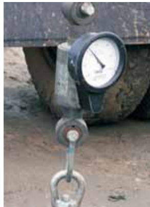
Helix Anchor Pulled-out at 50kN Load
