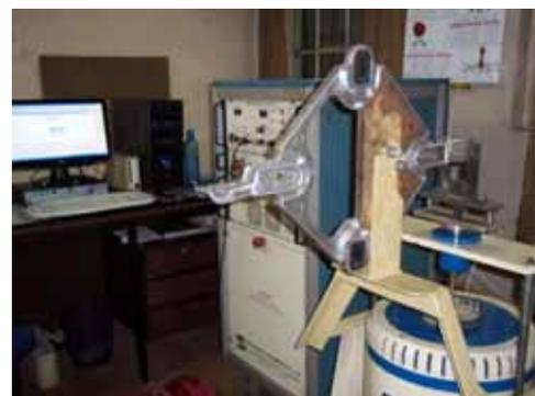
Testing of Quad Spacer Dampers
